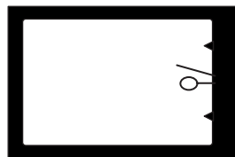
Match needle: correct exposure when two moving needles match up.
