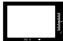
LED display: correct exposure when mark is positioned in the middle of the scale on the right.
